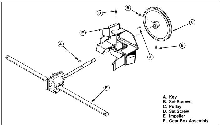
Figure 3. Auger Assembly
